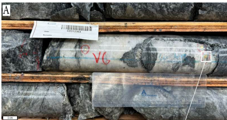
A .Representative specimens of the visible high grade gold VG discovered in the 25-DH-1286 hole in the K-Zone
